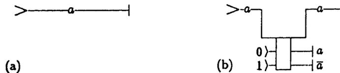
Figure 22. The value  $a$  carried by an arbitrary line (a) can be inspected in a nondestructive way by the "spy" device in (b).
