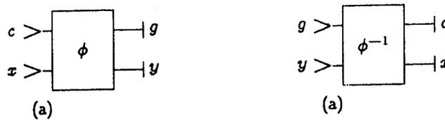
Figure 20. (a) Computation of  $y = f(x)$  by means of a combinational conservative-logic network  $\phi$ . (b) This computation is "undone" by the inverse network,  $\phi^{-1}$
